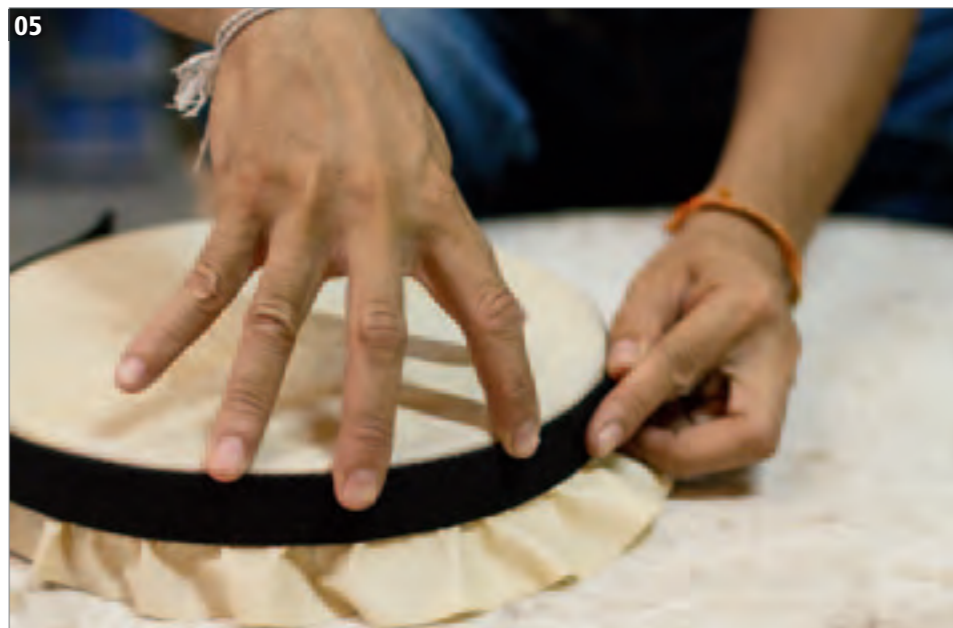
07 The head is tacked securely to the frame.
