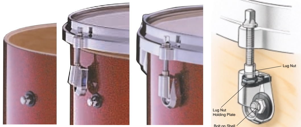
Air hole, YESS and bolts on the shell side are all positioned at the shell's nodal point.
